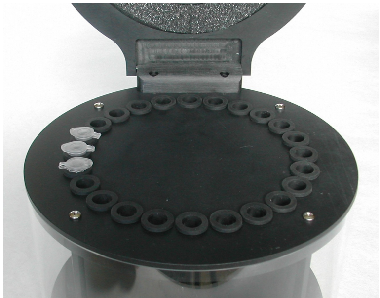
Two photos of the Bullet Blender™: the cover open (left) and a close up view showing 3 sample tubes in place (right).
