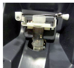
Homogenization of whole iris-ciliary body into 7mL vial with Minilys
