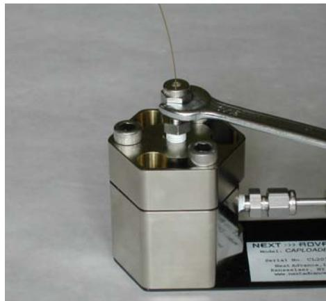
*Use a wrench to tighten the nut, forcing the ferrule to squeeze tightly around the capillary.*
