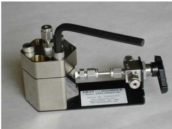
*Use a hex wrench to tighten the three bolts (shown on a different model pressure cell).*
