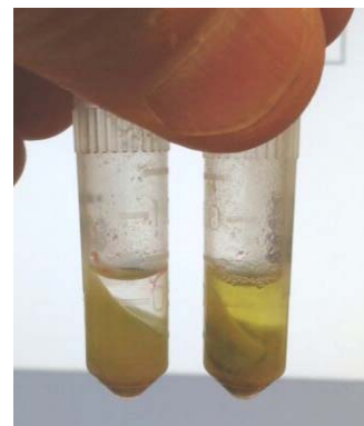
Figure 1. Comparison of supernatant from Synergy™ grinding media (left) to standard grinding media (right).
